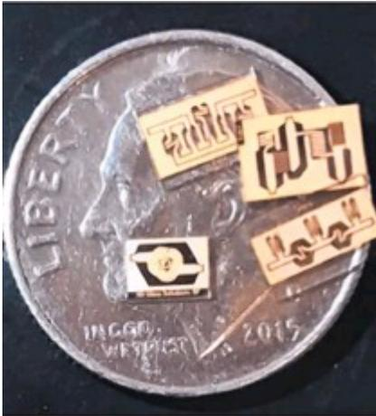
3D Glass has created a new process that uses ceramics to build glass circuit boards that can reduce the size of electronics packaging in everything from mobile devices to satellite communications by 70 percent, while using 50 percent less power than circuit boards used in most products today.
